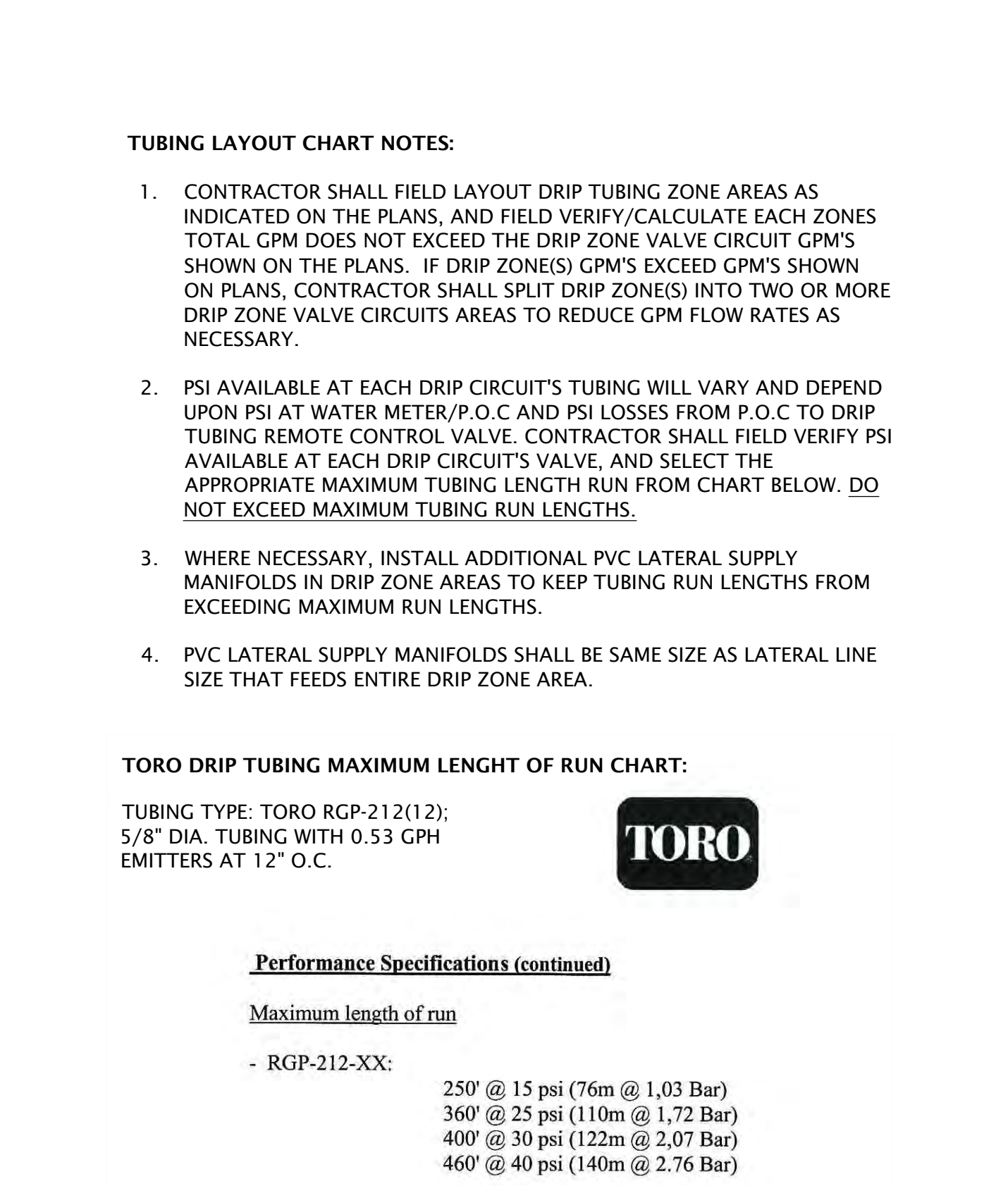
8 DRIP CIRCUIT MAXIMUM TUBING LENGTH CHART NOT TO SCALE
