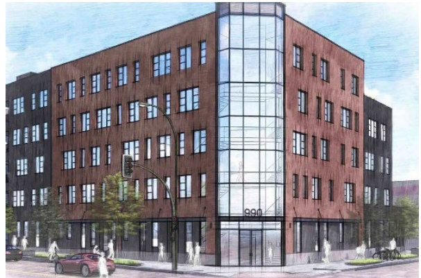
Chamfered corner entrance on corner building.
